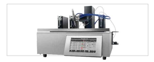
XYZ3000 3D platform dispenser adopts high-precision stepping pump to carry out liquid transportation, which can realize the control of non-pulse liquid flow and ensure the formation of uniform and single solution lines on the membrane. The instrument can not only carry out solution labeling to meet the requirements of the package of antibody solution of NC membrane in gold labeled strip, but also carry out solution spraying to meet the requirements of the package of gold spraying solution.
