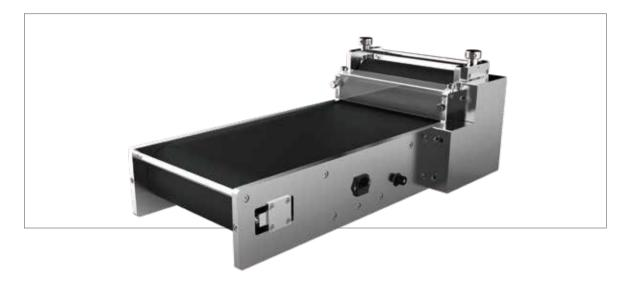
PSM200 assembly roller use mechanical compacting method to press and close the cassette firmly and quickly, it significantly reduces the labor force and increases the production efficiency. The running belt conveyors the semi-assembled cassettes to the rollers: one small prepress roller and a bigger compacting roller afterwards, after these twice pressing, the cassette can be closed perfectly. This instrument is widely used in rapid test production.
