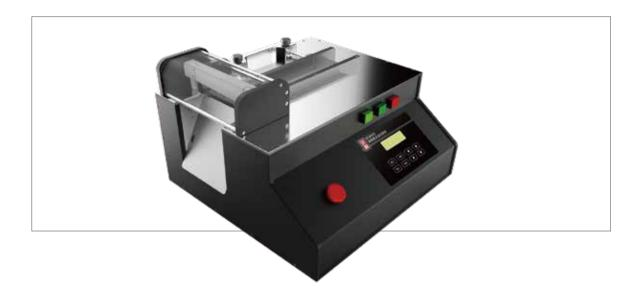
High Precision Strip Cutter adopts stepper motor to drive the mechanical parts to precisely control the inputting width of the sheet. This high speed and high torque motor drives blades along with the sheet feeding components to cut it into strips fast and accurately, it significantly reduces the labor cost and increase the work efficiency.
