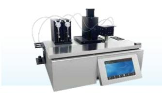
HMY300 dispenser instrument adopts high-precision stepping pump to carry out liquid transportation, which can realize the control of non-pulse liquid flow and ensure the formation of uniform and single solution lines on the membrane. The polyester hollow fiber tube used for dispensing has good strength and flexibility. When dispensing, it can not only ensure the quality of the line, but also ensure that the membrane surface structure is not damaged.
