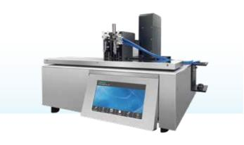
PJY200 high-precision 3D platform dispenser instrument adopts high-precision stepping pump to carry out liquid transportation, which can realize the control of non-pulse liquid flow and ensure the formation of uniform and single solution lines on the membrane. Gold spraying needs to be driven by the origin of external high pressure.
