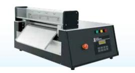
LCM Accessory cutter adopts the same principle as the strip guillotine cutter. The width of applicable cutting material is increased and it can used for sample pads, conjugate pads, absorbent pads, glass fiber and other pads.
