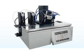
XYZ3000 3D platform dispenser adopts high-precision stepping pump to carry out liquid transportation, which can realize the control of non-pulse liquid flow and ensure the formation of uniform and single solution lines on the membrane. The instrument can not only carry out solution labeling to meet the requirements of the package of antibody solution of NC membrane in gold labeled strip, but also carry out solution spraying to meet the requirements of the package of gold spraying solution
